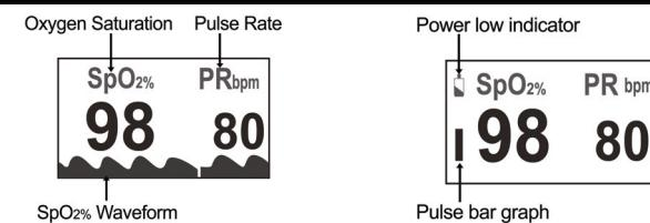
The height of the bar graph indicates of the pulse and signal strength. The bar should be greater than 30% for a proper reading.
